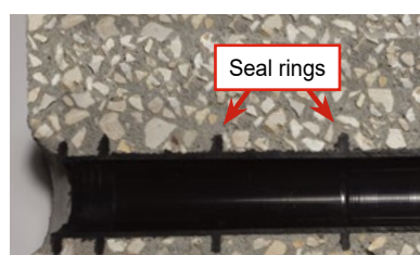
Pipe cut inside a concrete casting
