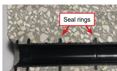
Pipe cut inside a concrete casting
